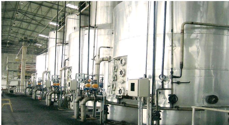
BATCH PANS WITH MECHANICAL CIRCULATOR
