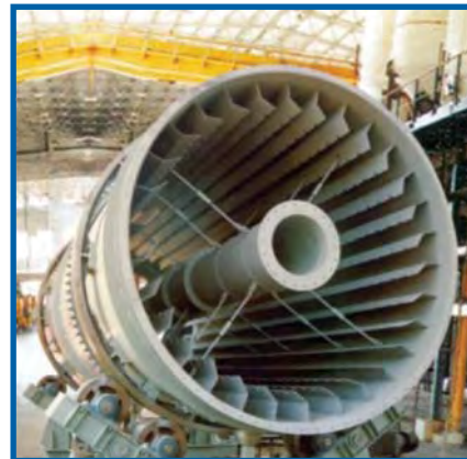
Rotary Sugar Drier (Capacity 10 tons/hr to 60 tons/hr)
