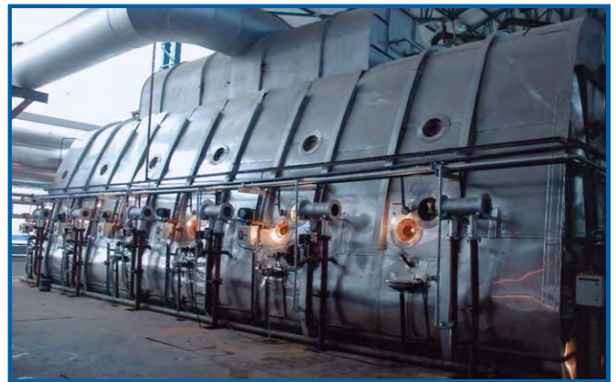
Continuous Vacuum Pan (Capacity Range 15 tons/hr to 150 tons/hr for High & Low Grade Masseccuite)
